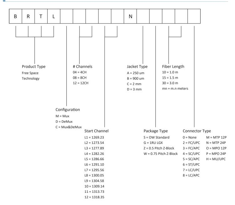
The characteristic of LWDM working wavelength is that it is located near zero dispersion, with small dispersion and good stability. At the same time, LWDM can support 12-wave 25G to increase the capacity and save fiber.
